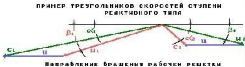
$$\alpha_1 = 12 \dots 22^\circ \quad \alpha_2 \rightarrow 90^\circ$$
