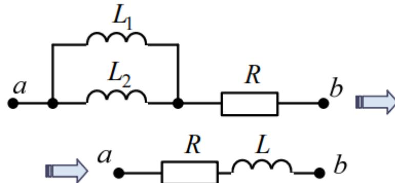
$$\text{здесь } R = R_1 + R_2; \quad L = \frac{L_1 \cdot L_2}{L_1 + L_2};$$
