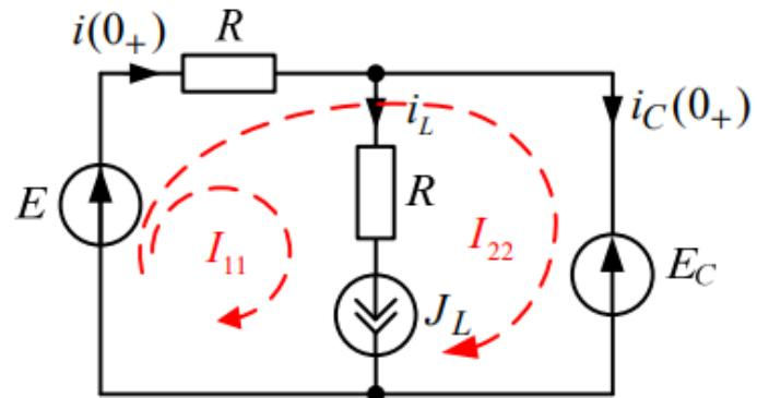
$$\begin{aligned} J_L &= i_L(0_-); \\ E_C &= u_C(0_-). \end{aligned}$$
