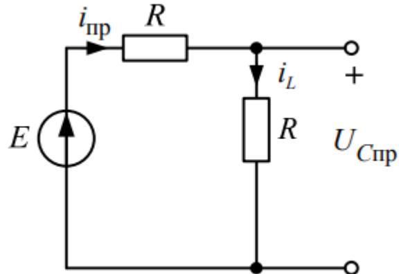
$$\begin{aligned} i_{\text{пр}} &= i_{L\text{пр}} = \frac{E}{2R} = 1,5 \text{ A}; \\ u_{C\text{пр}} &= R \cdot i_{L\text{пр}} = 150 \text{ В}; \\ i_{C\text{пр}} &= 0; \\ u_{L\text{пр}} &= 0. \end{aligned}$$
