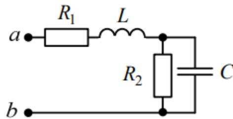
$$Z(p) = R_1 + pL + \frac{\frac{R_2}{pC}}{R_2 + \frac{1}{pC}}.$$
